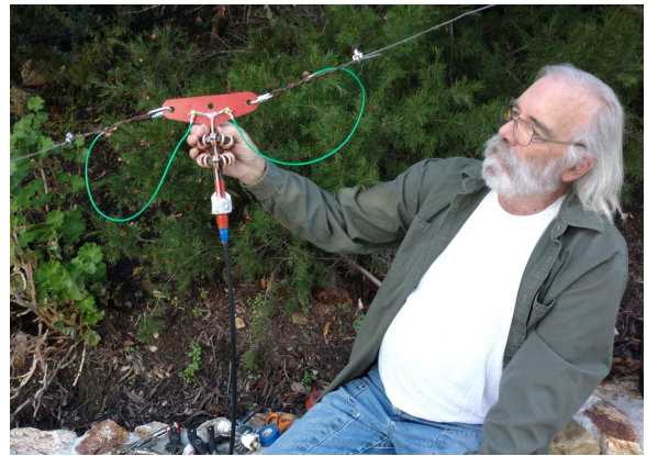
Fig 11 – W6GJB's Dipole Center Insulator With Two RG400 Chokes
